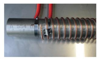
11 Image: Tightened wire connection clamp and hose clamp DN 100 as well as tightened hose connection clamp DN 100
