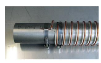
As is shown in images 10+11, the wire sits on the pipe and is fixed in place by the separate clamp, metal on metal. This type of connection is recommended. Other methods of grounding are also possible, however we would like to point out the following:
